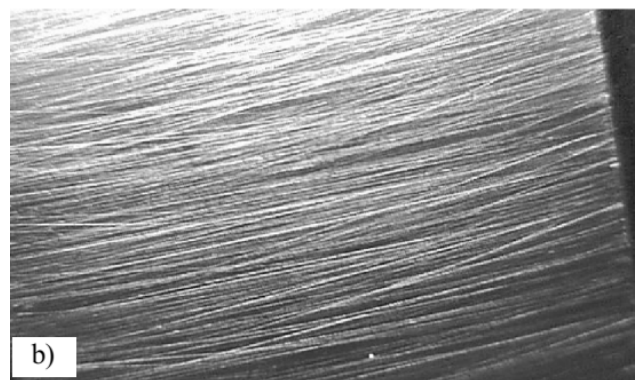
Figure. 3: (a) Abrasive wear on FIP plunger (b) Magnification x 10 (1)
