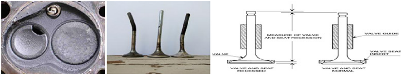
Figure 3. Failed exhaust valve due to high temperature corrosion (L), Fatigue (C), Recession (R)
