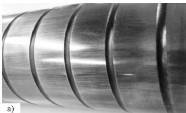
Figure. 3: (a) Abrasive wear on FIP plunger (b) Magnification x 10 (1)
