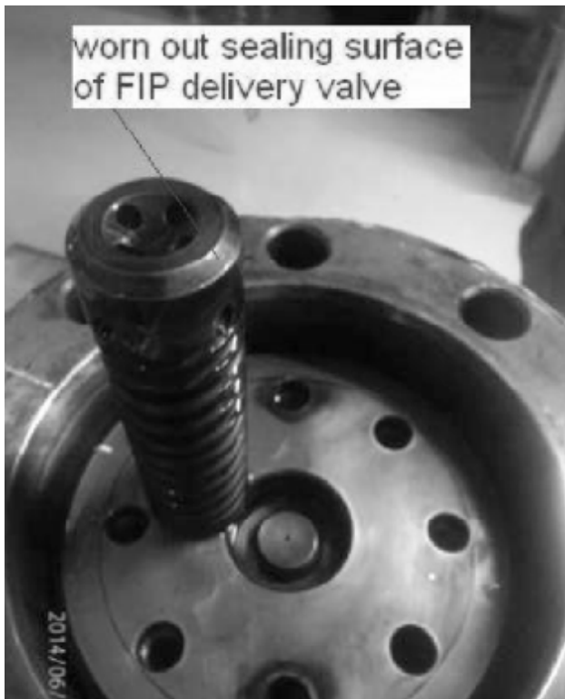
Figure. 8: Wear of delivery valve (1)
