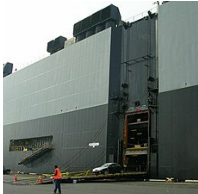
One of the Car Carriers with a Stbd side Side Ramp. Note Gangway and gangway space just aft of the Side ramp. Our main access door for cargo was very nearly similar to the above
