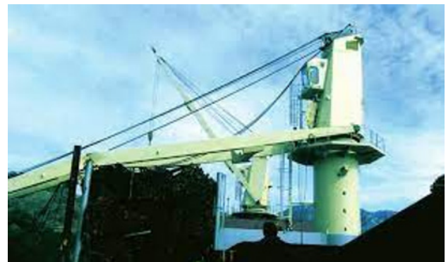
Courtesy picclub.or.jp // A damaged and bent jib // The bend of this jib is, comparatively, much less than the damage to our jib.
