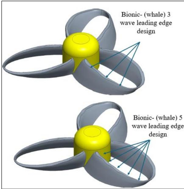
Fig. 8 Bionic toroidal propellers with 3 and 5 wave shape on leading edges
