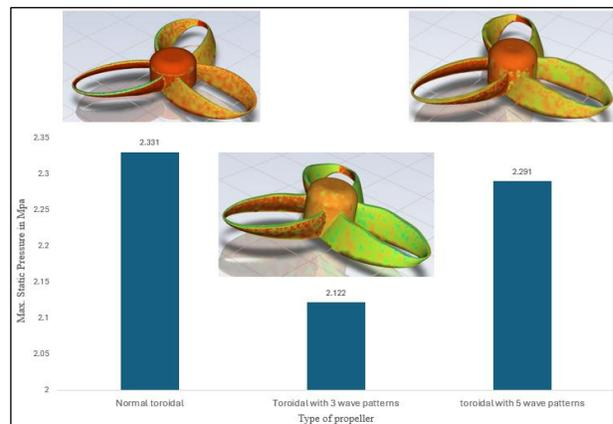
Fig. 14 Graph of Static pressures in different propellers
