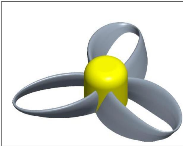
Fig. 6 Toroidal Propeller as a reference for analysis
