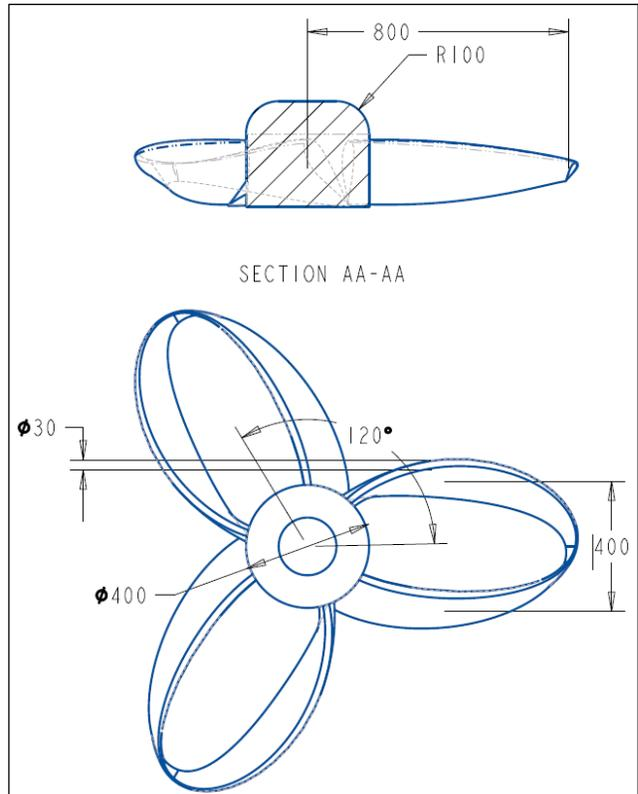
Fig. 7 Geometry of a Toroidal Propeller
