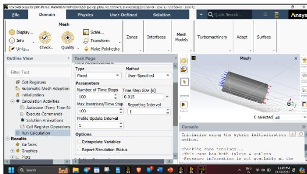
Fig. 12 Settings for time steps and iterations
