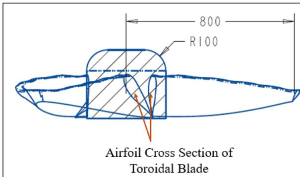
Fig. 9 Airfoil cross section of propeller blade
