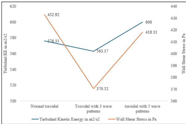
Fig. 15 graphs of TKE and wall shear for different propellers
