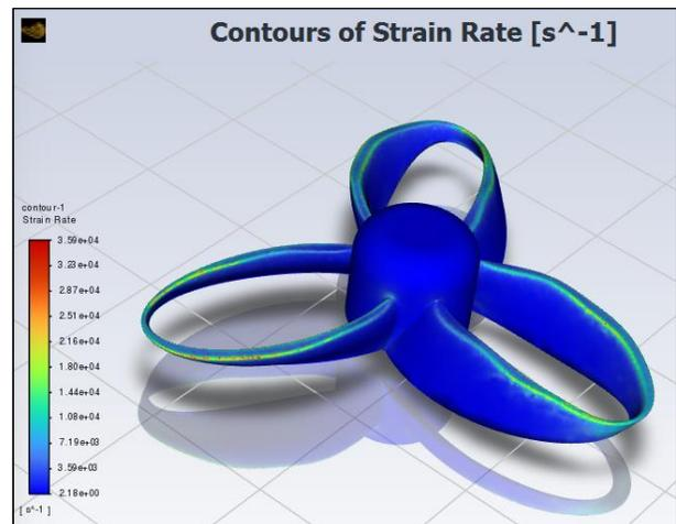
Fig. 17 Strain Rate of 3 wave pattern propeller
