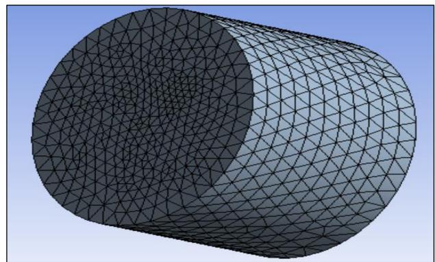
Fig. 11 Meshing (Nodes:202436, Elements: 1102580)
