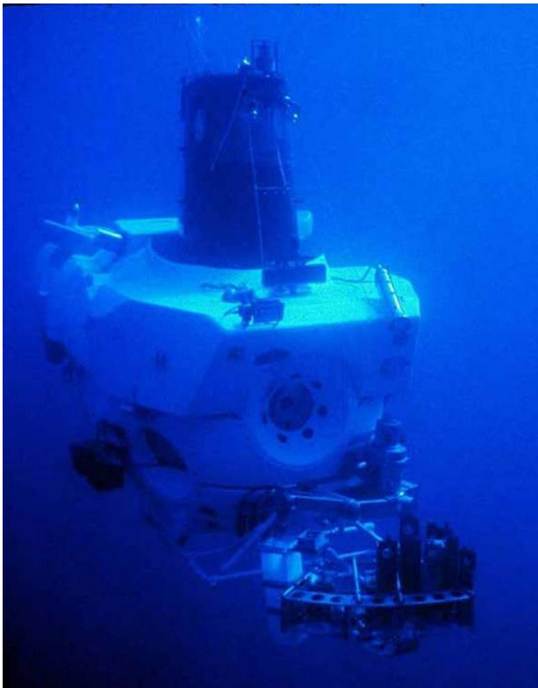
**←** *The DSV Alvin in 1978, exploring hyperthermal vents. The rack hanging at the bow holds sample containers*
