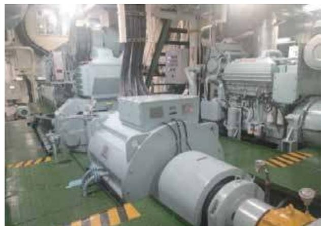
**Figure 8 – Actual Picture of Medium/High Speed shaft generator (courtesy – CSSC/SMDERI)**
