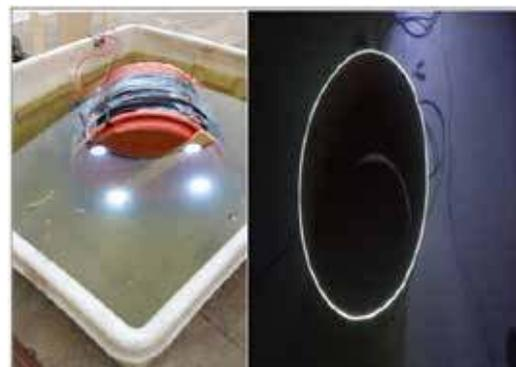
Figure 5. Dock with 4 LEDs (Type1) & circular strip LED (Type2)
