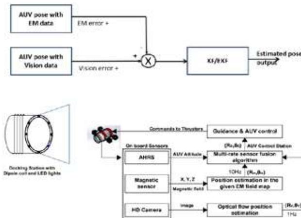
Figure 16. KF-based MSF algorithm for accurate attitude estimation
