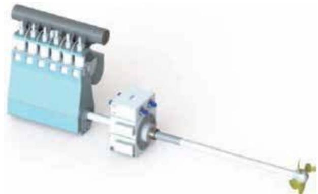
**Figure 3 – Schematic layout of low-speed type shaft generator - (courtesy – CSSC/SMDERI)**
