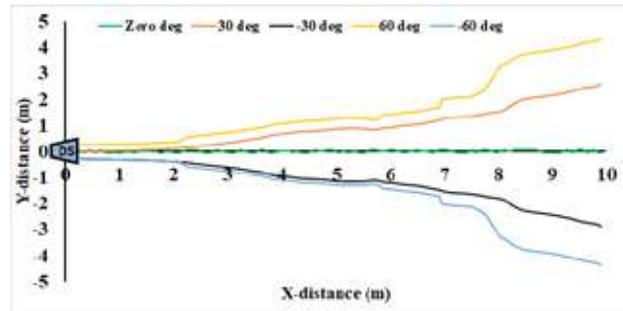
**Figure 14. Terminal position accuracy during BI-AUV homing**
