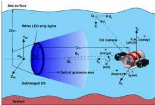
Figure 1. Concept of vision-based homing guidance
