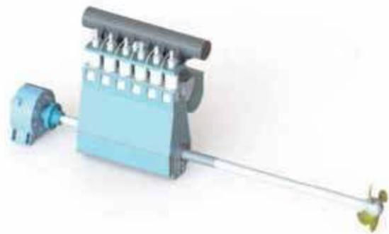
**Figure 4 – Schematic layout of Non Drive end type shaft generator. (courtesy – CSSC/SMDERI)**
