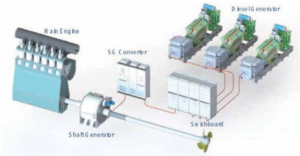
**Figure 10 - LAYOUT OF SHAFT GENERATOR SYSTEM**
