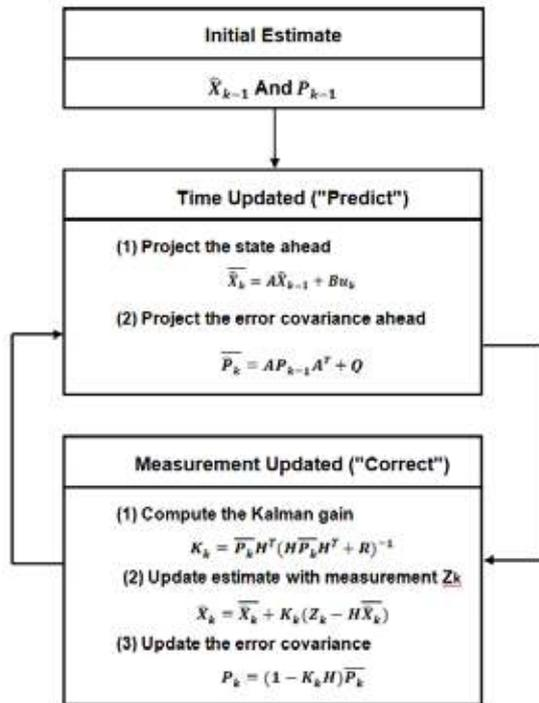
Figure 15. Principle of KF Algorithm
