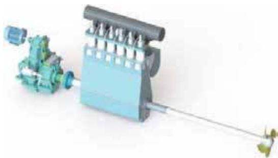
**Figure 5 – Schematic layout of Gear Type Shaft Generator (courtesy – CSSC/SMDERI)**
