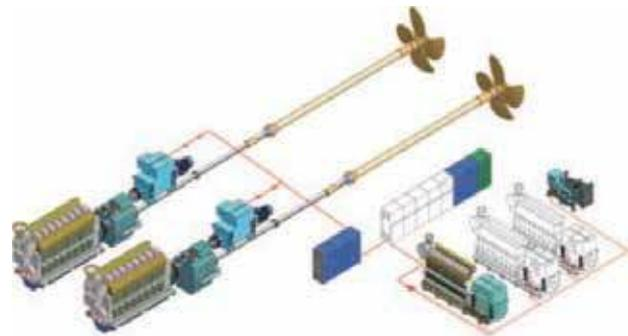
**Figure 7 – Schematic layout of Medium/High speed shaft Generator (courtesy – CSSC/SMDERI)**
