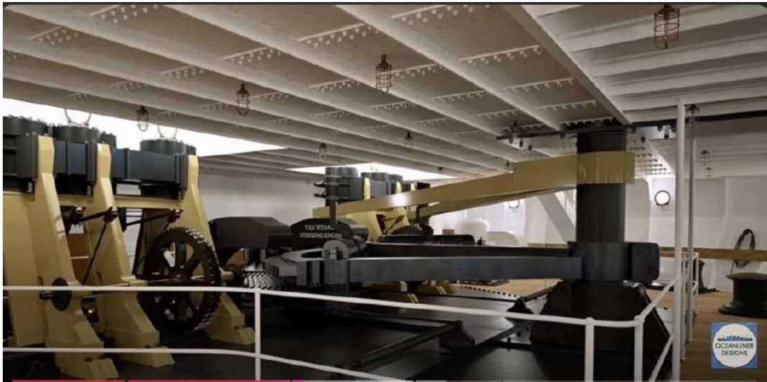
Titanic's Steering Gear for turning the rudder, located on C Deck
