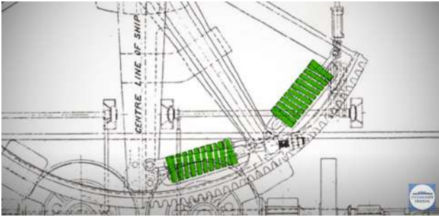
Heavy Duty Spring coils took up the shock of the turning of the heavy rudder
