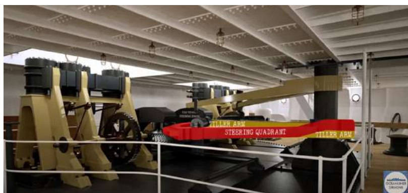
Tiller Arms were used to turn the rudder, to take up the load that would have, otherwise, come on the quadrant
